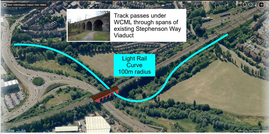
Possible alignment for a link between the Watford - St. Albans branch line on the east side of the WCML, and Overground networks on the west side.
